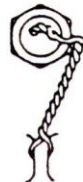
When Practical, hollow head plugs should be wired with the pigtail bent inside to avoid snags or injury
