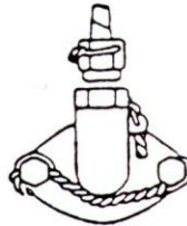
Bolt wired to a right angle bracket with the wire wrapped around the bracket
