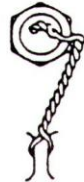
When Practical, hollow head plugs should be wired with the pigtail bent inside to avoid snags or injury
